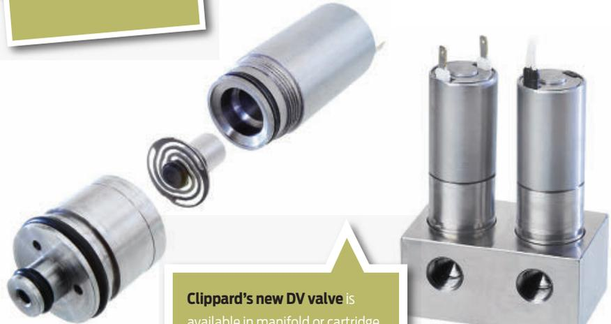
Clippard's new DV valve is available in manifold or cartridge styles, offering extremely high flow rates of 100 lpm at 100 psig.
